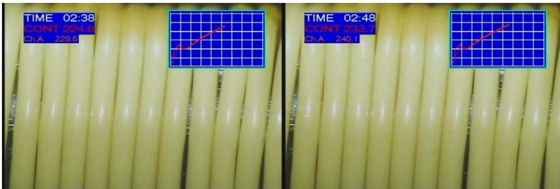
Photo3(a):TEX-E 0.20mm 230°C (bobbin 225°C) Photo3(b):TEX-E 0.20mm 240°C (bobbin 234°C)
