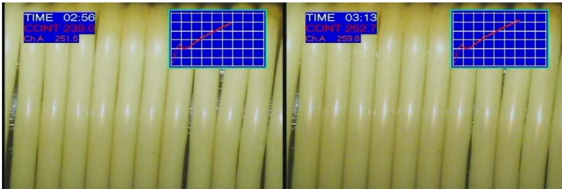
Photo3(c):TEX-E 0.20mm 251°C (bobbin 239°C) Photo3(d):TEX-E 0.20mm 260°C (bobbin 253°C)
